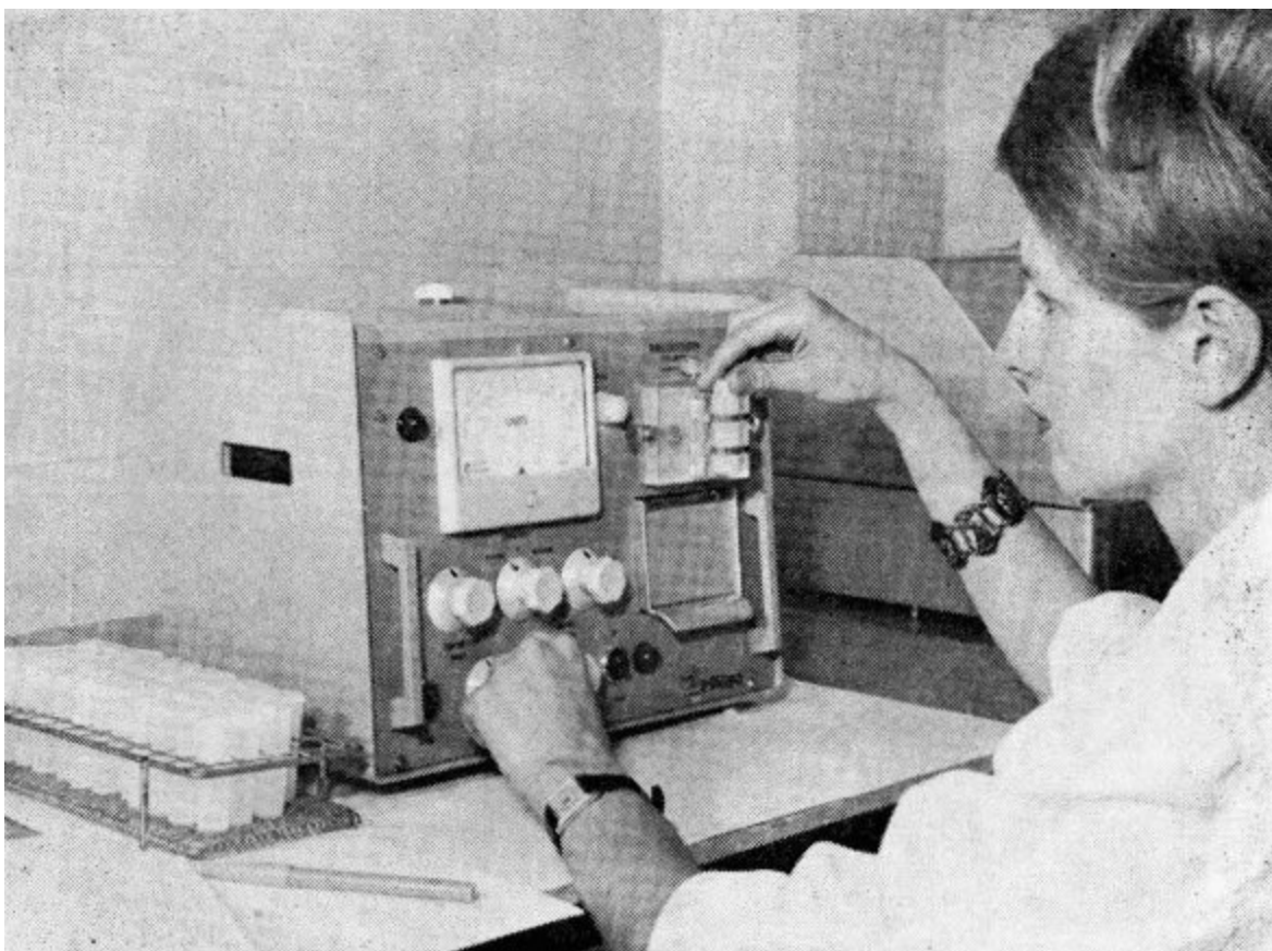
Figure 3. Oscillometric measurement of irradiated ampoules.
