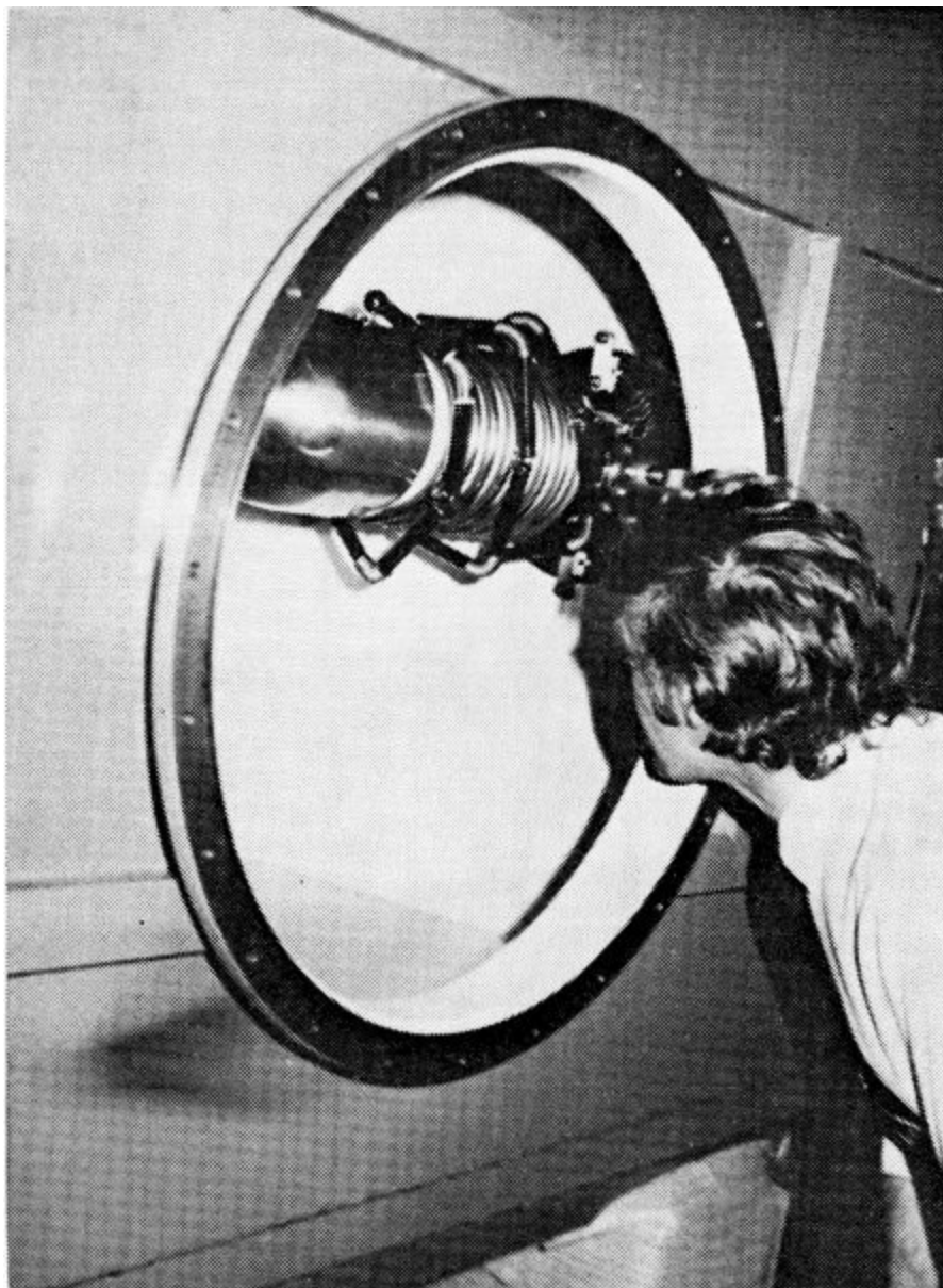
Figure 21. View of a 300kV, 2 Ampere Electron Gun Installed in the Injector Tank of a High Power 10MeV Linear Accelerator.
