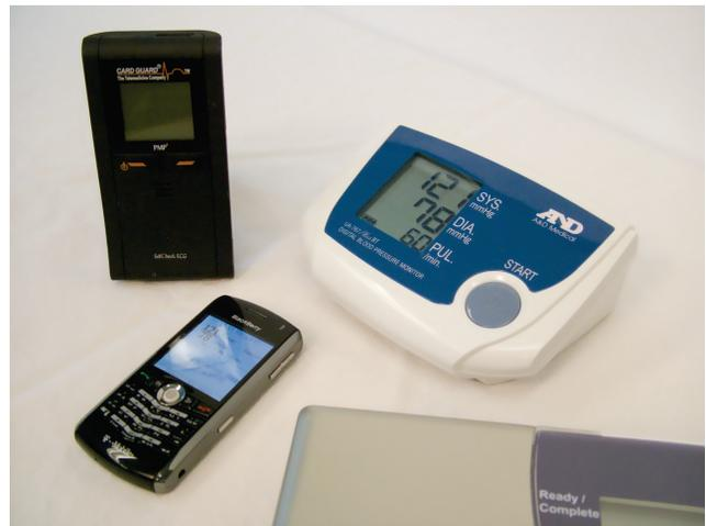
Figure 2. Mobile phone based remote patient monitoring. Bluetooth-enabled consumer medical devices connect to a patient’s mobile phone to facilitate self-care and clinical management of chronic conditions. Shown here are a Bluetooth-enabled single-lead ECG monitor, blood pressure monitor, and weight scale. A Java application on the mobile phone turns the device into a monitoring hub within the home, relaying data back to healthcare providers and returning instructions and advice to the patient.
