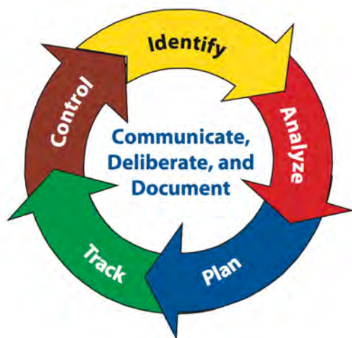
Figure 10. Continuous risk management. NASA and Steven Badelt. “Learning from Other Industries.” Presented at the AAMI/FDA Risk Management Summit, Sept. 29–30, 2015
