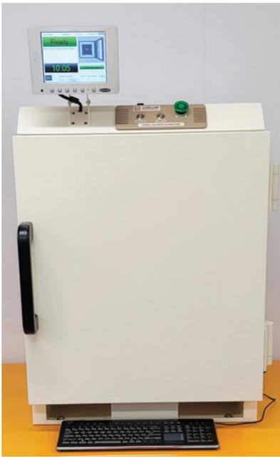
**Figure 5.** Ludlum Model 54A Small Article Monitor installed at STERIS Libertyville X-ray Radiation Technology Center. Image courtesy of STERIS.
