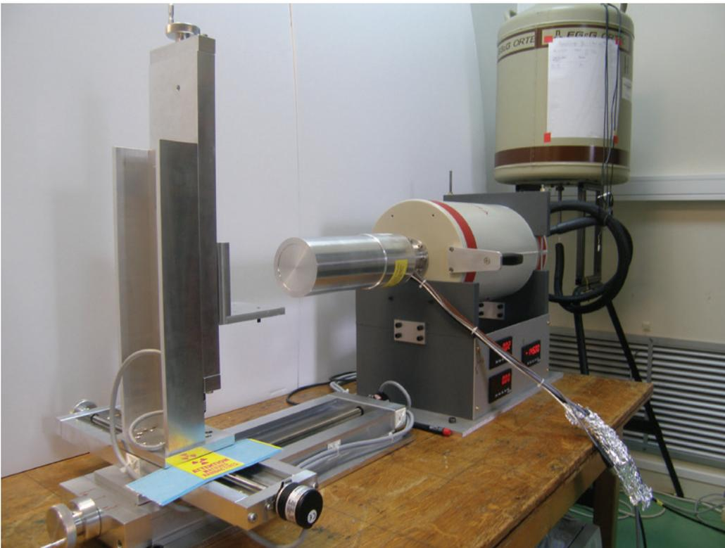
Figure 8. Germanium Hyper-Pure spectrometer. Image courtesy of STERIS.
