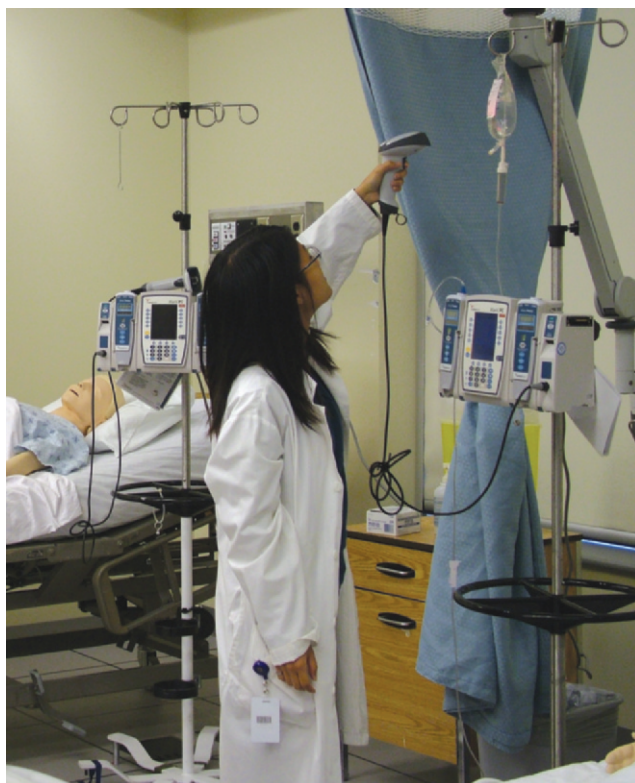
Figure 3. Nurse scans an IV bag drug label containing the patient name, drug name and concentration. This information is compared to the patient name scanned on the patient armband and if it matches, the drug and concentration are automatically selected during pump programming.
