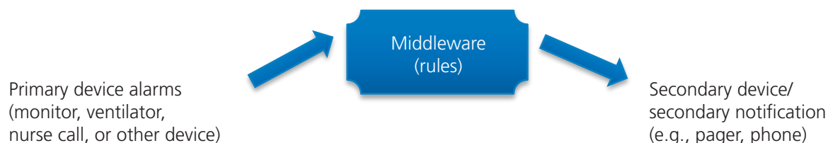
Figure 1. An alarm produced at a primary device flows through the middleware (software) to the secondary device for secondary alarm notification.
