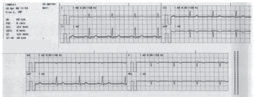
Figure 2. A) GE Solar 8000i monitor with <5k \Omega on all electrodes and peristaltic pump running. B) GE 8000i monitor with 100k \Omega on left leg, all other electrodes <5k \Omega , and peristaltic pump running.
