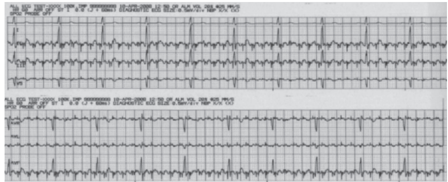
Figure 2. A) GE Solar 8000i monitor with <5k \Omega on all electrodes and peristaltic pump running. B) GE 8000i monitor with 100k \Omega on left leg, all other electrodes <5k \Omega , and peristaltic pump running.
