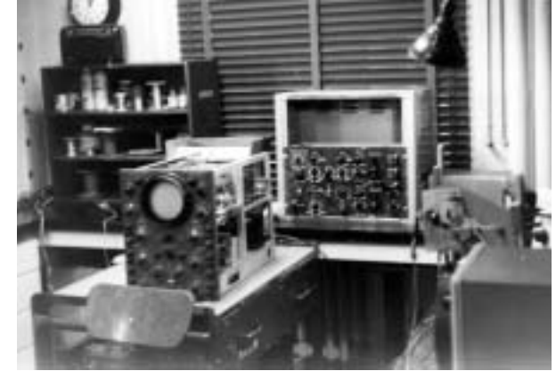
In this shot of Bill Staewen's biomedical shop in 1960, the equipment rack with an empty panel is an electromyograph he was building. It is used to analyze nerve and muscle activity.
