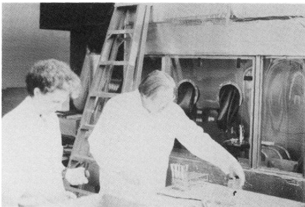
Figure 4. The Barrier Isolation Simulator which was Used to Perform Decontamination/Sterilization Studies
