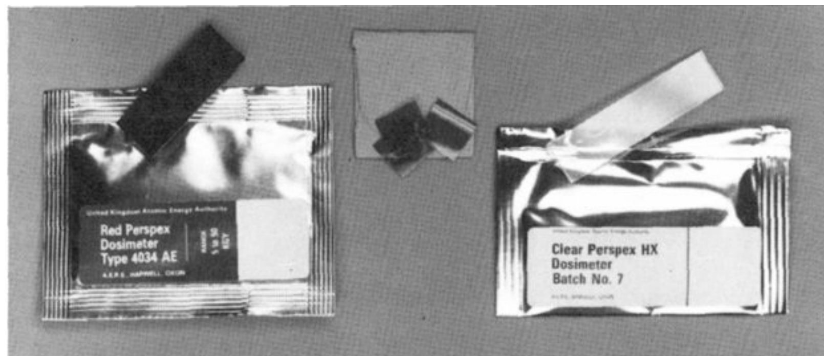
Figure 13. Routine Process-Monitoring Dosimeters
